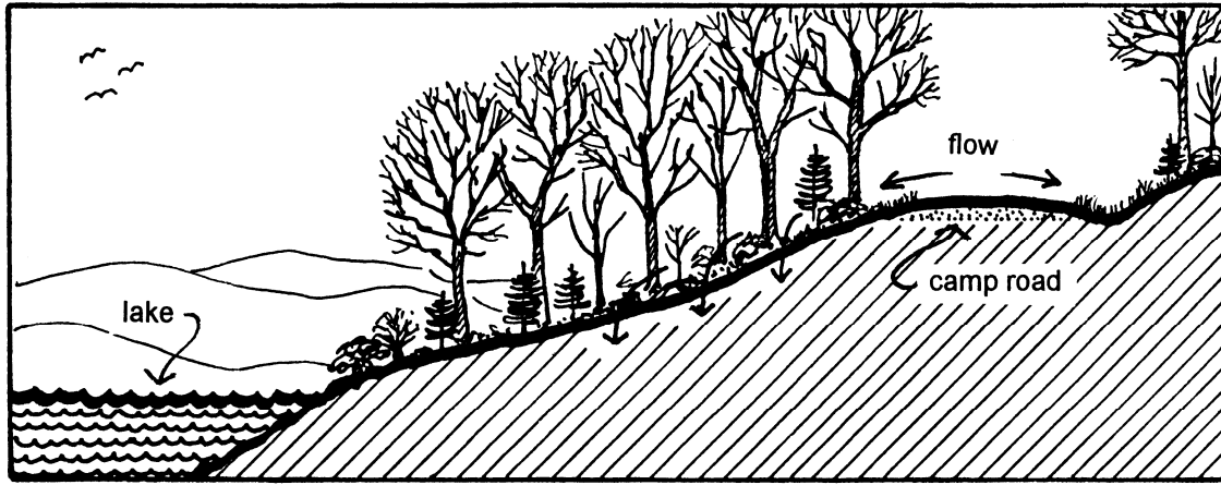
Figure 4. Vegetated buffers filter and absorb camp road runoff.
